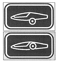
The landing gear is extended and retracted with the gray control handle located in the right hand armrest. Landing gear locked positions are located at either end of the control handle travel. Forward to extend, back to retract. The system is assisted by a nitrogen gas strut. See Maintenance Manual Section 2.
