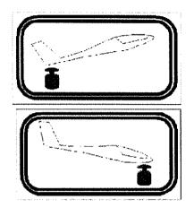
The trim adjustment control knob is located *in* the left armrest and controls the elevator trim select position. See Maintenance Manual Section 2. To set the trim, simply move the adjustment knob to the desired trim position.
